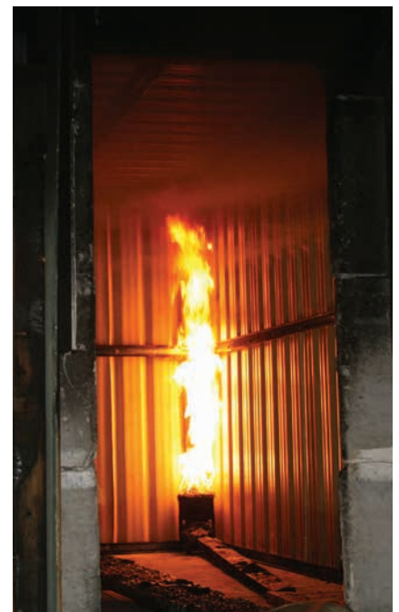
The full-scale ISO 9705 Room Test
