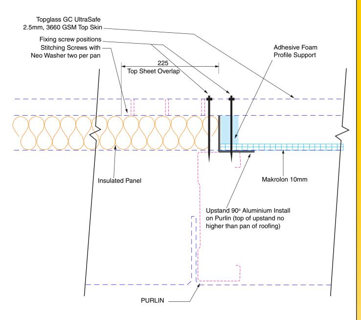
Thermal Product Testing carried out at AWTA Testing laboratories on the Alsynite Tripleskin Roofing System confirms a Means R Value of 0.57.
