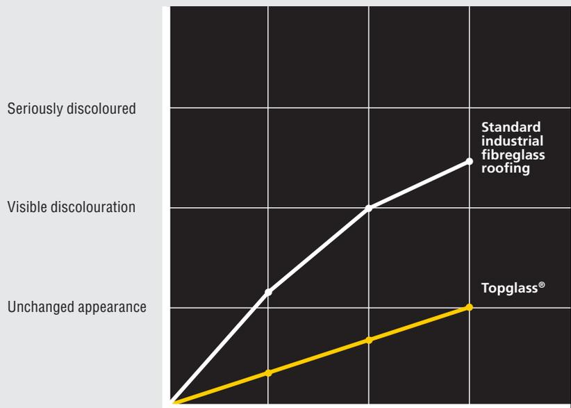
4,000 hours weatherometer testing simulates 10 years exposure in normal conditions
