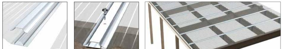
Now the sheet is ready to be laid on the roof with the lap connector. Predrill the 12mm oversize hole and Screw down into the rafters or purlins as required.
